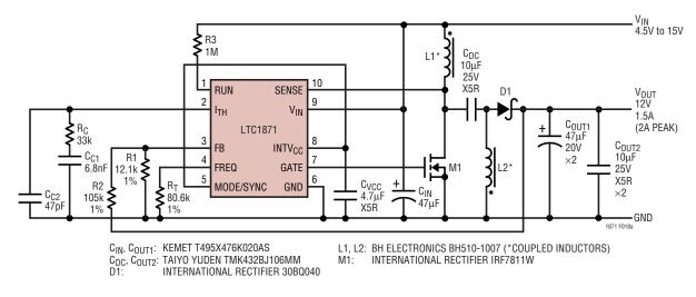
Figure 18a. 4.5V to 15V Input, 12V/2A Output SEPIC Converter
