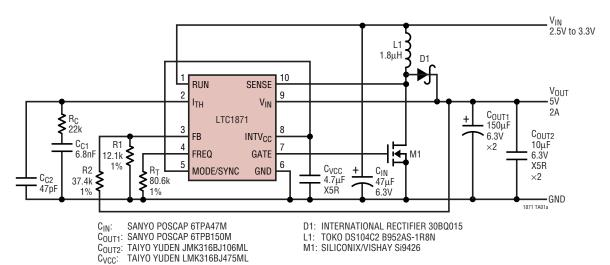
2.5V to 3.3V Input, 5V/2A Output Boost Converter
