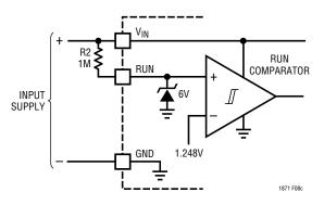
Figure 8c. External Pull-Up Resistor On RUN Pin for "Always On" Operation
