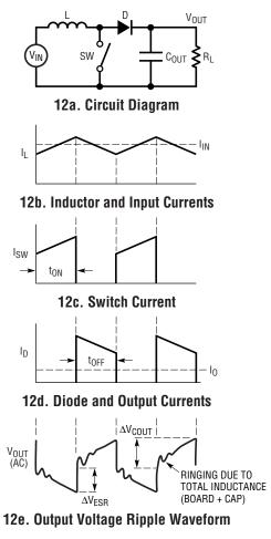
Figure 12. Switching Waveforms for a Boost Converter
