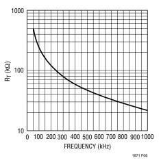
Figure 6. Timing Resistor (R<sub>T</sub>) Value
