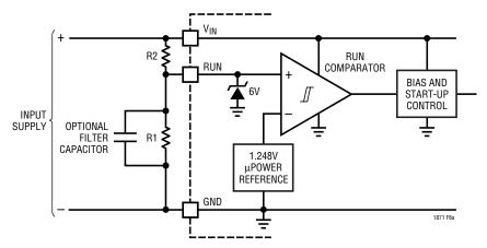
Figure 8a. Programming the Turn-On and Turn-Off Thresholds Using the RUN Pin
