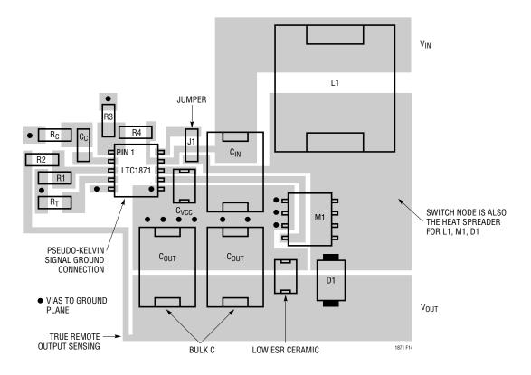
Figure 14. LTC1871 Boost Converter Suggested Layout
