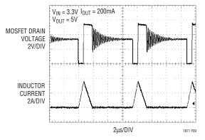
Figure 9. Discontinuous Mode Waveforms
