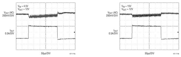
Figure 19. LTC1871 SEPIC Converter Load Step Response
