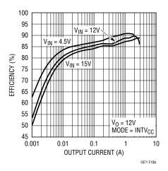
Figure 18b. SEPIC Efficiency vs Output Current
