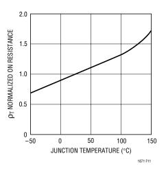
Figure 11. Normalized R<sub>DS(ON)</sub> vs Temperature
