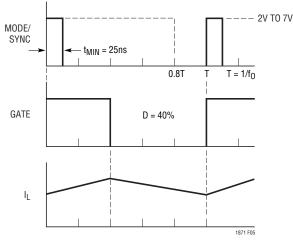
Figure 5. MODE/SYNC Clock Input and Switching Waveforms for Synchronized Operation
