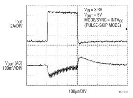
Figure 13. Load Transient Response for a 3.3V Input, 5V Output Boost Converter Application, 0.7A to 7A Step
