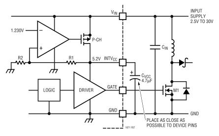
Figure 7. Bypassing the LDO Regulator and Gate Driver Supply
