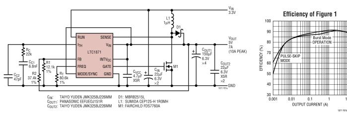
Figure 1. High Efficiency 3.3V Input, 5V Output Boost Converter (Bootstrapped)
