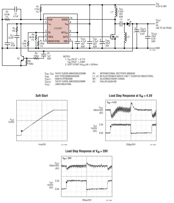
4.5V to 28V Input, 5V/2A Output SEPIC Converter with Undervoltage Lockout and Soft-Start
