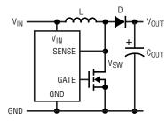
2a. SENSE Pin Connection for Maximum Efficiency (V<sub>SW</sub> < 36V)
