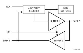
Figure 3. Simplified Block Diagram of the Digital Data Transfer Operation
