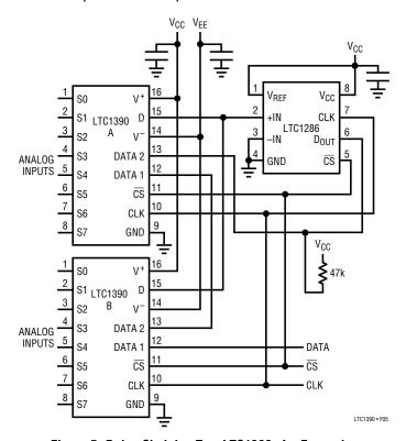
Figure 5. Daisy-Chaining Two LTC1390s for Expansion
