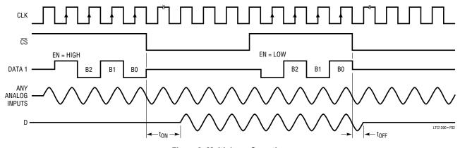
Figure 2: Multiplexer Operation
