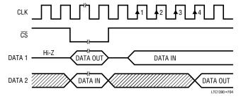
Figure 4. Digital Data Transfer Operation
