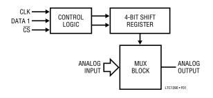
Figure 1: Simplified Block Diagram of the MUX Operation
