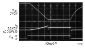
Figure 9.  $R_{SS}$  = 15k,  $C_{SS}$  = 68nF;  $V_{OUT}$  Reaches –5V in 1.6ms; Input Current Peaks at 350mA
