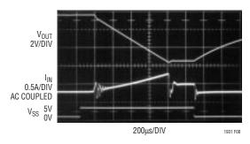
Figure 8.  $R_{SS}$  = 15k,  $C_{SS}$  = 33nF;  $V_{OUT}$  Reaches –5V in 1ms; Input Current Peaks at 500mA
