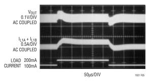
Figure 5. Transient Response of Inverting Converter with 22 $\mu$ F Tantalum Output Capacitor and No Phase Lead Capacitor
