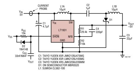
Figure 7. R<sub>SS</sub> and C<sub>SS</sub> at SHDN Pin Provide Soft-Start to LT1931 Inverting Converter
