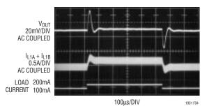
Figure 4. Transient Response of Inverting Converter with 220pF Phase Lead Capacitor
