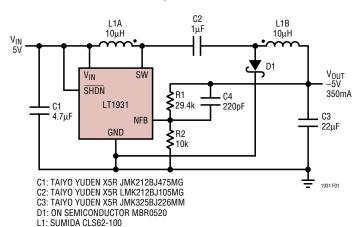
Figure 1. 5V to -5V, 350mA Inverting DC/DC Converter
