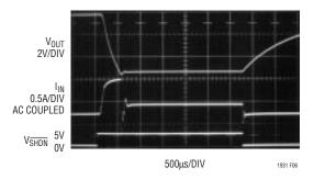
Figure 6. Start-Up Waveforms for 5V to -5V Application (Figure 1). No Soft-Start Circuit. V<sub>OUT</sub> Reaches -5V in 500µs; Input Current Peaks at 800mA
