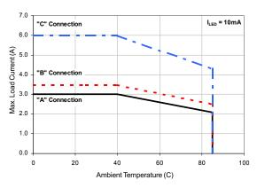
Figure 1.Typical Current Derating Curves\*
