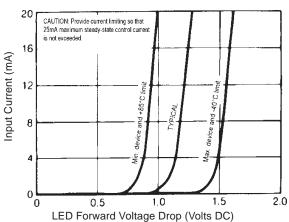
Figure 6. Input Characteristics (Current Controlled)
