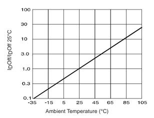
Figure 5. Normalized Off-State Leakage
