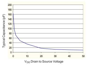
Figure 9. Typical Output Capacitance
