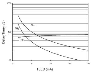
Figure 7. Typical Delay Times
