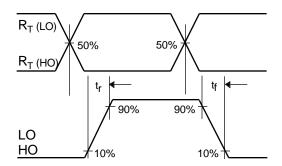
Figure 1. Input/Output Timing Diagram
