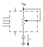
Two terminal Variable Resistor; Variable current
