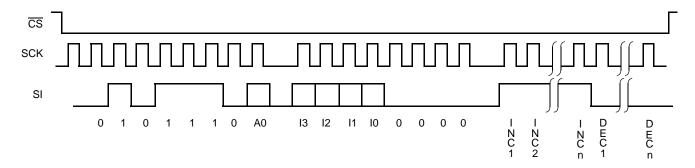
**Figure 8. Increment/Decrement Timing Limits**
