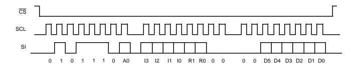
Figure 6. Three-Byte Instruction Sequence (Read)
