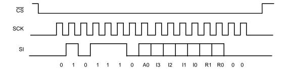
Figure 5. Three-Byte Instruction Sequence (Write)
