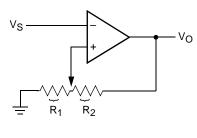
$$\begin{aligned} &V_{UL} = \{R_1/CR_1 + R_2\} \ V_O(max) \\ &V_{LL} = \{R_1/CR_1 + R_2\} \ V_O(min) \end{aligned}$$
