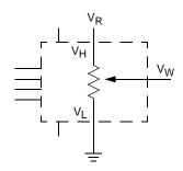
Three terminal Potentiometer; Variable voltage divider
