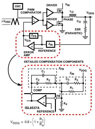
FIGURE 3. VOLTAGE-MODE BUCK CONVERTER
