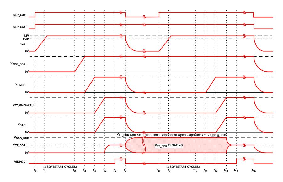
FIGURE 1. ISL6537A TIMING DIAGRAM
