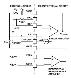
FIGURE 5. OUTPUT VOLTAGE AND LOAD-LINE
