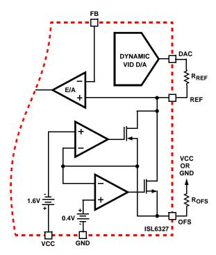
FIGURE 6. OUTPUT VOLTAGE OFFSET PROGRAMMING
