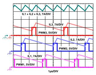
FIGURE 1. PWM AND INDUCTOR-CURRENT WAVEFORMS
