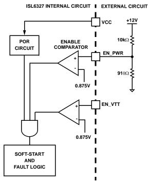
FIGURE 7. POWER SEQUENCING USING THRESHOLD-SENSITIVE ENABLE (EN) FUNCTION
