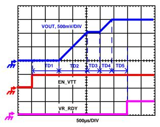
FIGURE 8. SOFT-START WAVEFORMS
