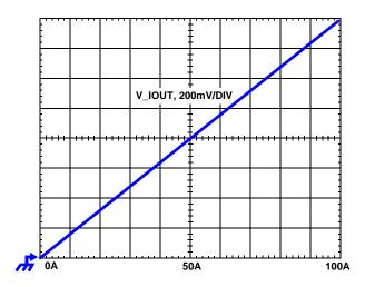
FIGURE 11. VOLTAGE AT IOUT PIN WITH A NTC NETWORK
