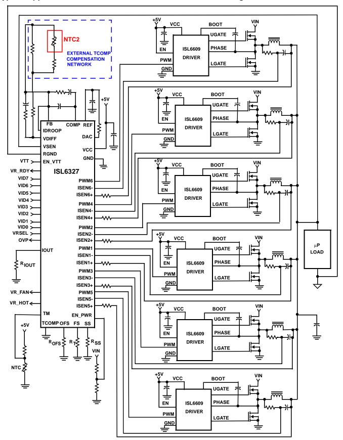
Typical Application - 6-Phase Buck Converter with DCR Sensing and Integrated TCOMP
