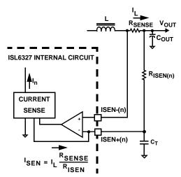
FIGURE 4. SENSE RESISTOR IN SERIES WITH INDUCTORS
