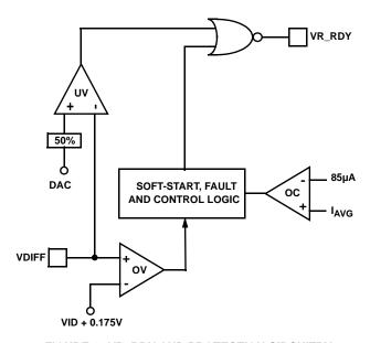
FIGURE 9. VR\_RDY AND PROTECTION CIRCUITRY
