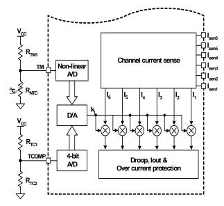
FIGURE 15. BLOCK DIAGRAM OF INTEGRATED TEMPERATURE COMPENSATION
