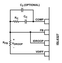
FIGURE 17. COMPENSATION CONFIGURATION FOR **LOAD-LINE REGULATED ISL6327 CIRCUIT**
