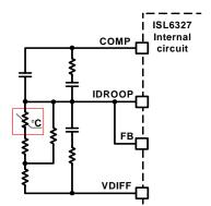
FIGURE 16. EXTERNAL TEMPERATURE COMPENSATION
