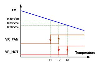
FIGURE 14. VR\_HOT AND VR\_FAN SIGNAL vs TM VOLTAGE
