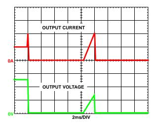
FIGURE 10. OVERCURRENT BEHAVIOR IN HICCUP MODE.  $F_{SW} = 500 \text{kHz}$
