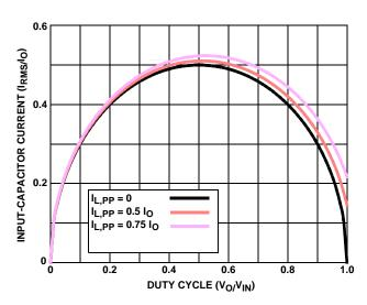
FIGURE 22. NORMALIZED INPUT-CAPACITOR RMS
