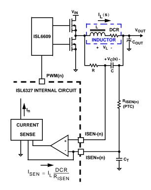
FIGURE 3. DCR SENSING CONFIGURATION
