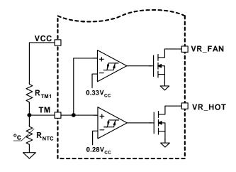
FIGURE 12. BLOCK DIAGRAM OF THERMAL MONITORING FUNCTION
