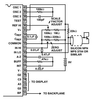
A silicon diode-connected transistor has a temperature coefficient of about  $\,\text{-}2\text{mV}/^{\text{O}}\text{C}$ . Calibration is achieved by placing the sensing transistor in ice water and adjusting the zeroing potentiometer for a 000.0 reading. The sensor should then be placed in boiling water and the scale-factor potentiometer adjusted for a 100.0 reading.
