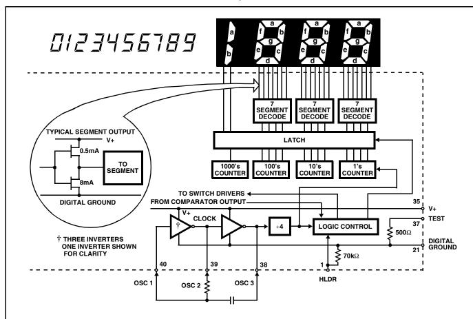
FIGURE 8. ICL7117 DIGITAL SECTION
