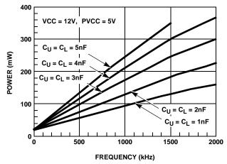
FIGURE 4. POWER DISSIPATION vs FREQUENCY (HIP6603B)
