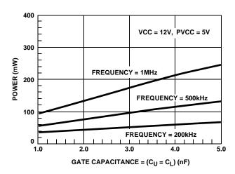
FIGURE 6. VARIABLE LOADING PROFILE (HIP6603B)
