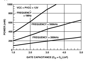
FIGURE 3. POWER DISSIPATION vs LOADING
