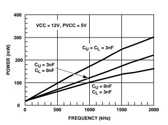
FIGURE 5. 3nF LOADING PROFILE (HIP6603B)
