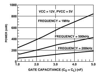
FIGURE 7. POWER DISSIPATION vs FREQUENCY (HIP6601B)
