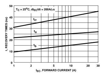
FIGURE 18. RECOVERY TIME vs FORWARD CURRENT
