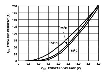
FIGURE 17. DIODE FORWARD CURRENT vs FORWARD VOLTAGE DROP
