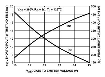
FIGURE 4. SHORT CIRCUIT WITHSTAND TIME
