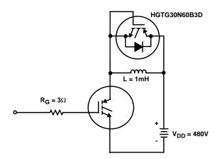
FIGURE 19. INDUCTIVE SWITCHING TEST CIRCUIT
