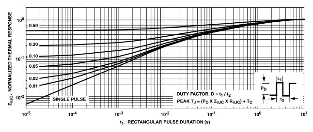
FIGURE 16. NORMALIZED TRANSIENT THERMAL RESPONSE, JUNCTION TO CASE
