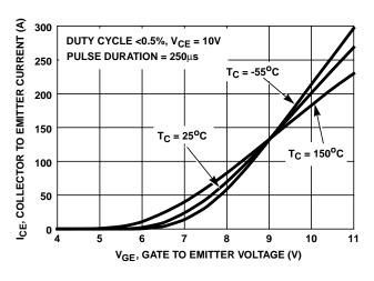
FIGURE 13. TRANSFER CHARACTERISTIC
