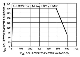
FIGURE 2. MINIMUM SWITCHING SAFE OPERATING AREA
