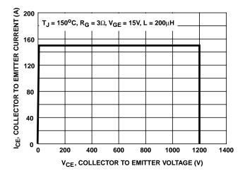
FIGURE 2. MINIMUM SWITCHING SAFE OPERATING AREA
