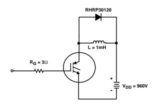
FIGURE 18. INDUCTIVE SWITCHING TEST CIRCUIT
