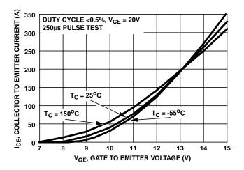
FIGURE 13. TRANSFER CHARACTERISTIC
