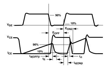
FIGURE 19. SWITCHING TEST WAVEFORMS
