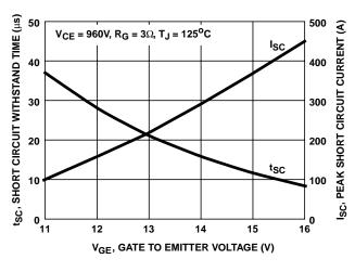
FIGURE 4. SHORT CIRCUIT WITHSTAND TIME
