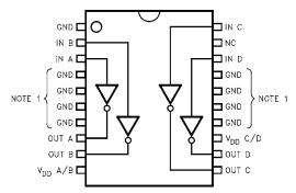
Note 1: Pins 4-7 and 14-17 are electrically connected.
