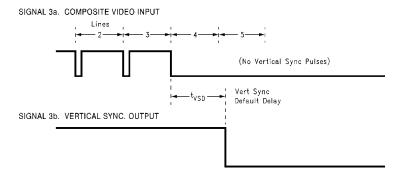
FIGURE 14. NON-STANDARD VERTICAL TIMING
