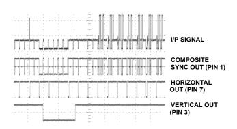
FIGURE 16. EXAMPLE OF EL1883 WITH NTSC SIGNAL THAT INCLUDES MACROVISION COPY PROTECTION ( $R_{SET}$ =681 $k\Omega$ )
