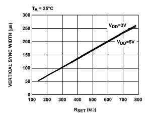
FIGURE 5. VERTICAL SYNC WIDTH vs R<sub>SET</sub>
