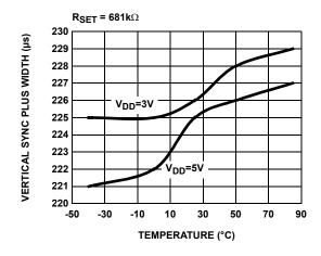
FIGURE 9. VERTICAL SYNC PULSE WIDTH vs TEMPERATURE
