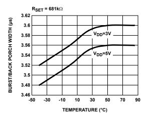
FIGURE 8. BURST/BACK PORCH WIDTH vs TEMPERATURE
