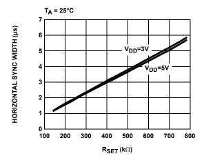
FIGURE 3. HORIZONTAL SYNC WIDTH vs R<sub>SET</sub>
