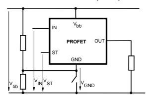
Any kind of load. If  $V_{GND} > V_{IN} - V_{IN(T+)}$  device stays off Due to  $V_{GND} > 0$ , no  $V_{ST} = low$  signal available.
