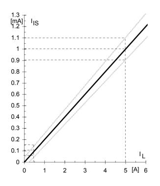
This range for the current sense ratio refers to all devices. The accuracy of the  $k_{\rm ILIS}$  can be raised at least by a factor of two by matching the value of  $k_{\rm ILIS}$  for every single device.
