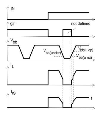
Figure 6b: Undervoltage restart of charge pump
