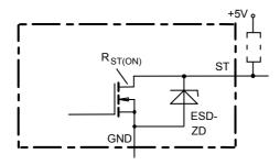
ESD-Zener diode: 6.1 V typ., max 5.0 mA;  $R_{ST(ON)}$  < 375  $\Omega$  at 1.6 mA. The use of ESD zener diodes as voltage clamp at DC conditions is not recommended.
