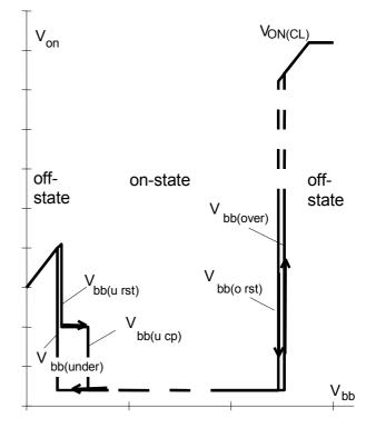
charge pump starts at  $V_{bb(ucp)} = 4.7 \text{ V typ.}$
