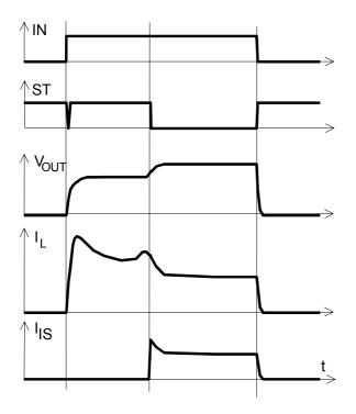
Figure 2d: Switching an inductive load
