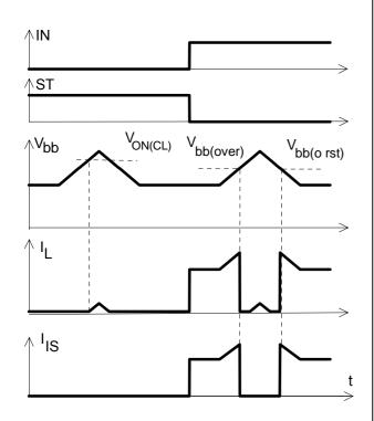
Figure 8a: Current sense versus load current<sup>26</sup>::
