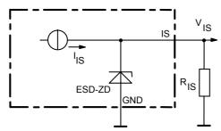
ESD-Zener diode: 6.1 V typ., max 14 mA;  $R_{IS} = 1 \text{ k}\Omega \text{ nominal}$
