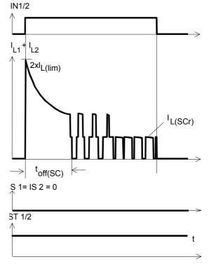
ST1 and ST2 have to be configured as a 'Wired OR' function ST1/2 with a single pull-up resistor.
