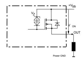
$V_{ON}$  clamped to  $V_{ON(CL)} = 47 \text{ V typ.}$
