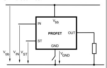
Any kind of load. In case of IN = high is  $V_{OUT} \approx V_{IN} - V_{IN}(T+)$ . Due to  $V_{GND} > 0$ , no  $V_{ST} = low$  signal available.
