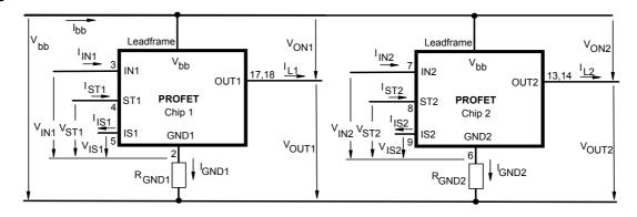
Leadframe (V<sub>bb</sub>) is connected to pin 1,10,11,12,15,16,19,20
