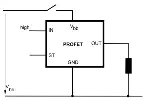
For inductive load currents up to the limits defined by  $Z_{\rm L}$  (max. ratings and diagram on page 10) each switch is protected against loss of  $V_{bb}$ .
