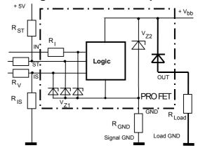
$V_{Z1}$  = 6.1 V typ.,  $V_{Z2}$  = 47 V typ.,  $R_{GND}$  = 150 Ω,  $R_{ST}$ =15kΩ,  $R_{I}$ =4.5kΩ typ.,  $R_{IS}$ =1kΩ,  $R_{V}$ =15kΩ, In case of reverse battery the current has to be limited by the load. Temperature protection is not active
