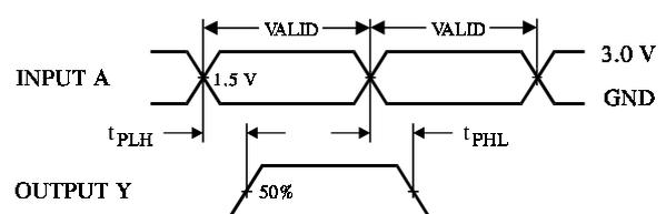
Figure 2. Switching Waveform
