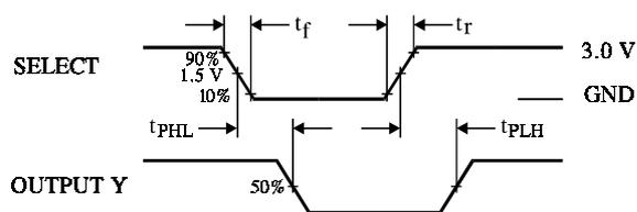
Figure 1. Switching Waveform
