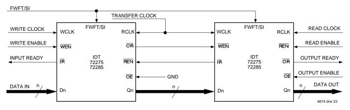
Figure 20. Block Diagram of 65,536 x 18 and 131,072 x 18 Depth Expansion
