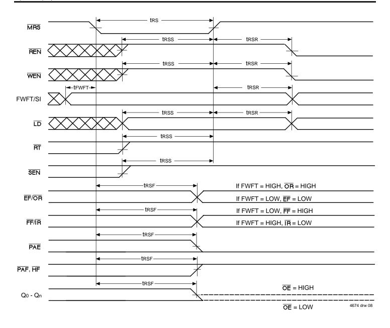
Figure 5. Master Reset Timing
