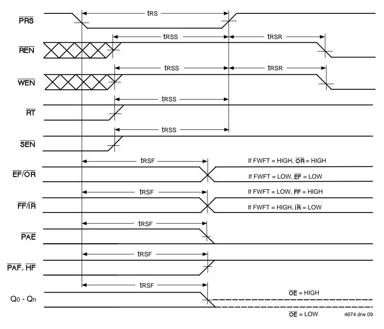
Figure 6. Partial Reset Timing
