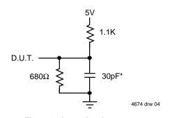
Figure 2. Output Load \* Includes jig and scope capacitances.
