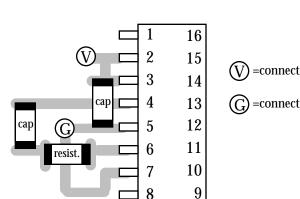
(V) =connect to VDD (G) =connect to GND
