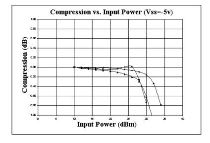
The P1dB curve shows all states with a P1dB compression at approximately 31dB input power. The conditions for this curve are Vdd = +5.0v and Vss = -5.0v.
