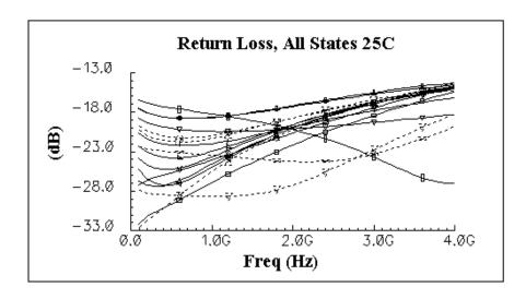
This Return Loss set of curves represents the combination of all Return Loss cases for all attenuation settings. All cases are better than -14dB Return Loss at 4GHz.
