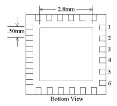
This package conforms to the LPCC<sup>TM</sup> 4 X 4 mm 24 lead body dimensions. See ASAT LPCC Marketing Outline Dwg. # DGMJ00004 Latest Rev. at <a href="http://www.asat.com">http://www.asat.com</a> for additional dimensional information.
