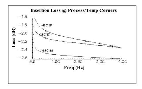
This Insertion Loss curve represents the Min/Max conditions for the "0" pass state versus all processing and temperature conditions. The Min case is at -40C with the "Fast" processing conditions. The Max case is at +85C with the "Slow" processing conditions. All other combinations fall within that band. The typical 25C case is labeled +25C TT.
