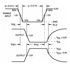
FIGURE 2. AC Waveforms
