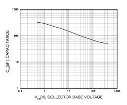
Figure 3. Collector Output Capacitance
