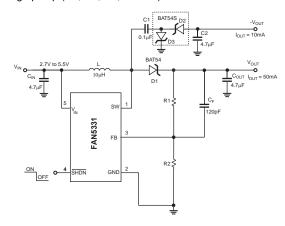
Figure 7. Dual (±) Boost Converter
