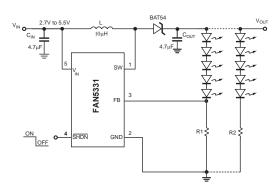
Figure 6. Low Noise Boost LED Driver
