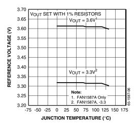
Figure 5. Output Voltage vs. Temperature
