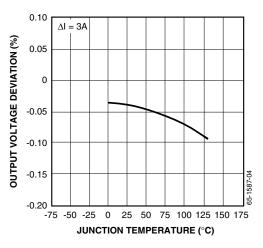
Figure 3. Load Regulation vs. Temperature
