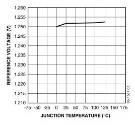
Figure 4. Reference Voltage vs. Temperature
