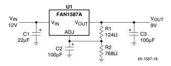
Figure 15. Application Circuit (FAN1587A)
