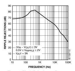
Figure 9. Ripple Rejection vs. Frequency
