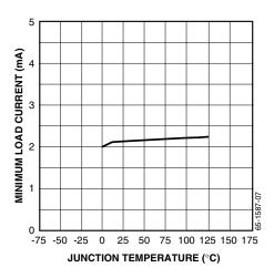
Figure 6. Minimum Load Current vs. Temperature
