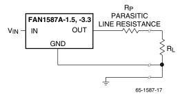
Figure 13. Connection for Best Load Regulation
