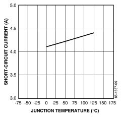
Figure 8. Short-Circuit Current vs. Temperature
