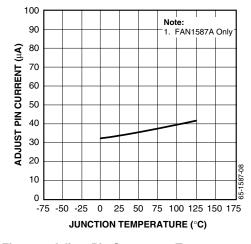
Figure 7. Adjust Pin Current vs. Temperature
