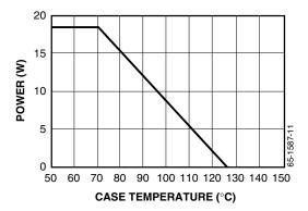
Figure 10. Maximum Power Dissipation
