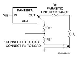
Figure 14. Connection for Best Load Regulation
