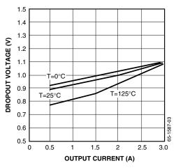
Figure 2. Dropout Voltage vs. Output Current
