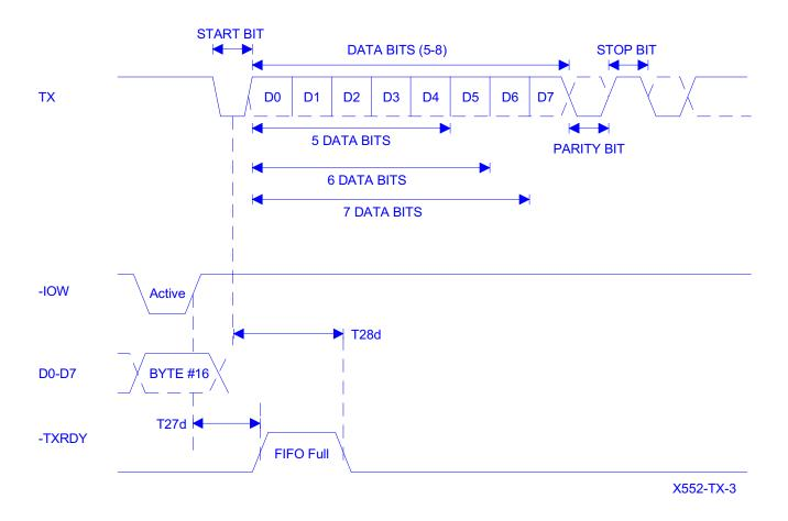
Transmit ready timing in FIFO mode
