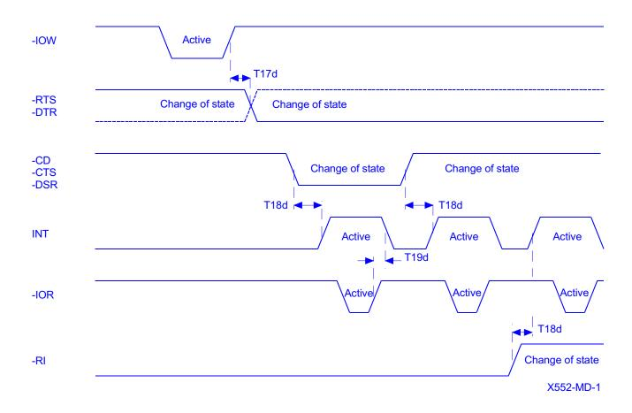
Modem input/output timing
