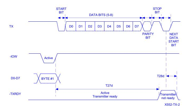
Transmit ready timing in none FIFO mode
