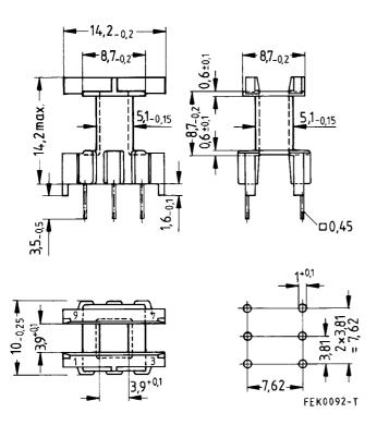
Hole arrangement View in mounting direction
