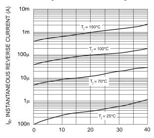
V<sub>R</sub>, INSTANTANEOUS REVERSE VOLTAGE (V) Fig. 3 Typical Reverse Current vs. Reverse Voltage
