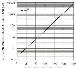
T<sub>J</sub>, JUNCTION TEMPERATURE (°C) Fig. 4 Typical Reverse Current vs. Junction Temperature
