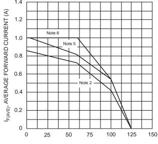
T<sub>A</sub>, AMBIENT TEMPERATURE (°C) Fig. 1 Forward Current Derating
