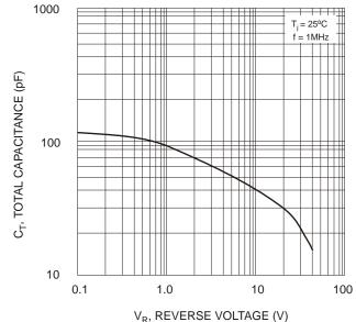
Fig. 5 Typical Total Capacitance vs. Reverse Voltage
