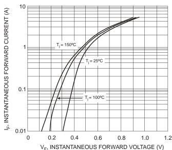
V<sub>F</sub>, INSTANTANEOUS FORWARD VOLTAGE (V) Fig. 2 Typical Forward Characteristics
