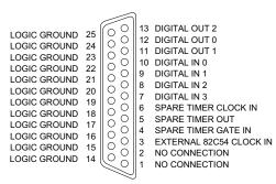
Figure 3. Digital I/O Connector - P4
