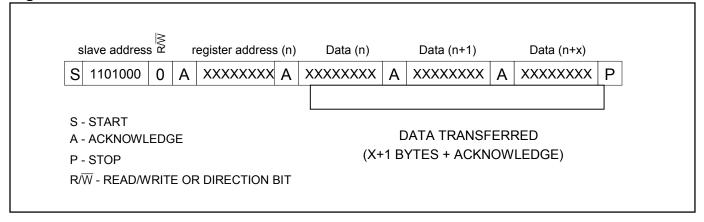
Figure 9. Data Read—Slave Transmitter Mode
