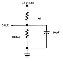
\* INCLUDING SCOPE AND JIG CAPACITANCE
