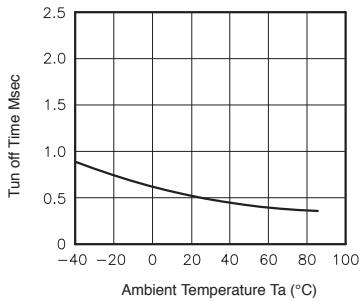
**Fig.5** LED operate vs. ambient temperature
