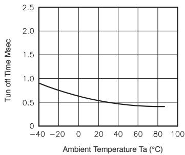
**Fig.5** LED operate vs. ambient temperature
