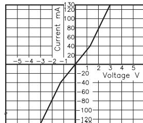
**Fig.9** Off state leakage current
