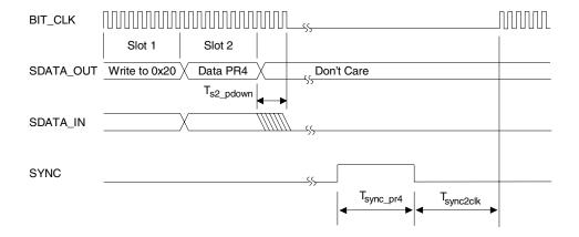
Figure 5. PR4 Powerdown and Warm Reset
