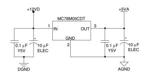
Figure 32. +5V Analog Voltage Regulator
