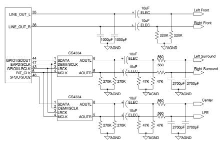
Figure 15. Serial Data Port: Six Channel Circuit
