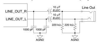
Figure 31. Stereo Output
