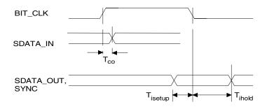
Figure 4. Data Setup and Hold
