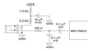
Figure 28. Microphone Input
