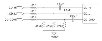
Figure 27. Differential 1  $V_{RMS}$  CD Input
