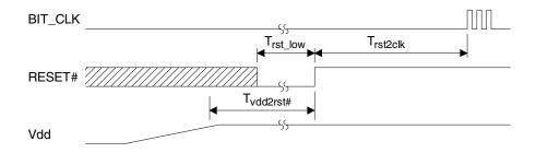
Figure 1. Power Up Timing
