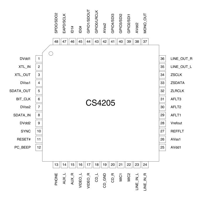
Figure 34. Pin Locations for the CS4205
