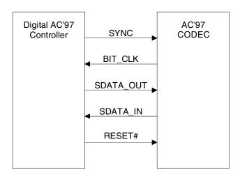
Figure 7. AC-link Connections
