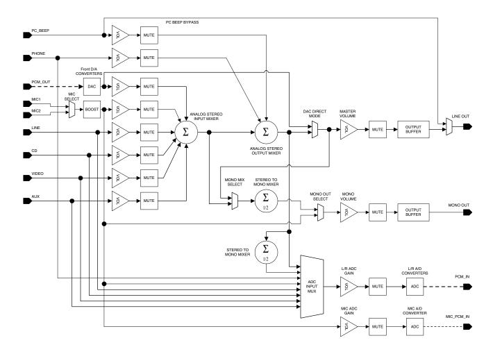
Figure 8. CS4205 Mixer Diagram
