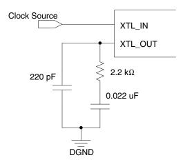
Figure 23. PLL External Loop Filter
