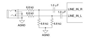
Figure 25. Line Input (Replicate for Video and AUX)
