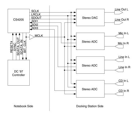
Figure 16. Digital Docking Connection Diagram
