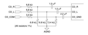
Figure 26. Differential 2 V<sub>RMS</sub> CD Input
