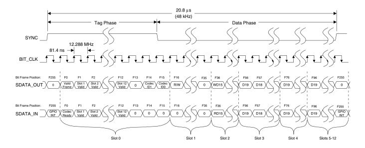
Figure 14. AC-link Input and Output Framing
