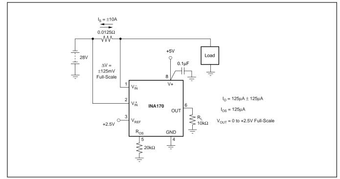
FIGURE 5. Bipolar Current Measurement.
