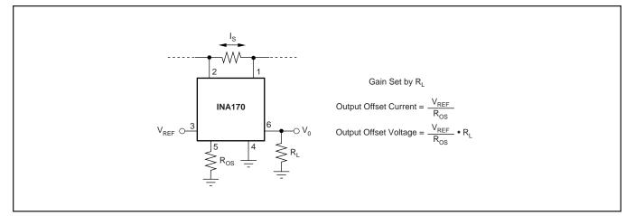
FIGURE 4. Offsetting the Output Voltage.
