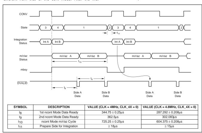
Figure 13. Non-Continuous Mode Timing
