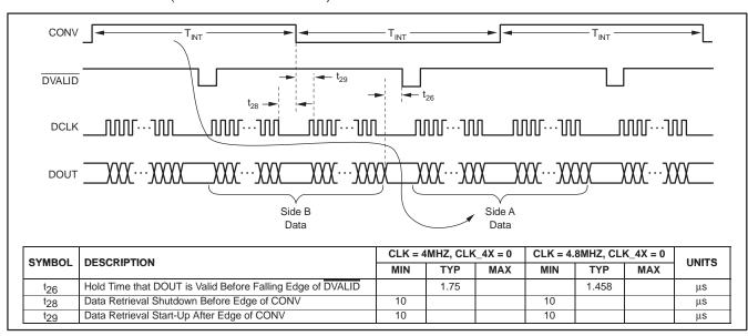
Figure 25. Readback Before and After CONV Toggles
