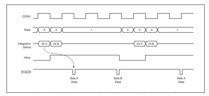
Figure 17. Non-Continuous Mode Timing with a 50% Duty Cycle CONV Signal
