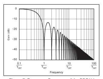
Figure 7. Frequency Response of the DDC114
