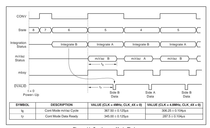
Figure 11. Continuous Mode Timing
