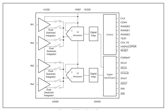
Figure 1. DDC114 Block Diagram
