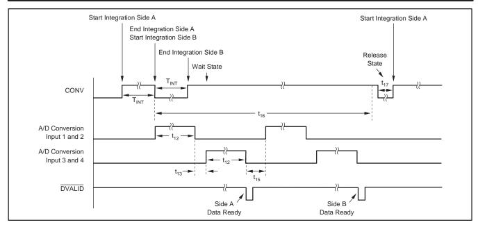
Figure 14. Conversion Detail for the Internal Operation of the Non-Continuous Mode with Side A Integrated First
