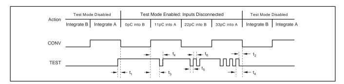
Figure 8. Timing Diagram of the Test Mode of the DDC114
