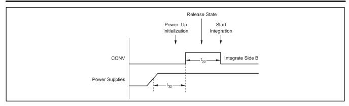
Figure 27. Timing Diagram at Power-Up of the DDC114
