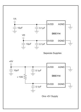
Figure 28. Power-Supply Connection Options
