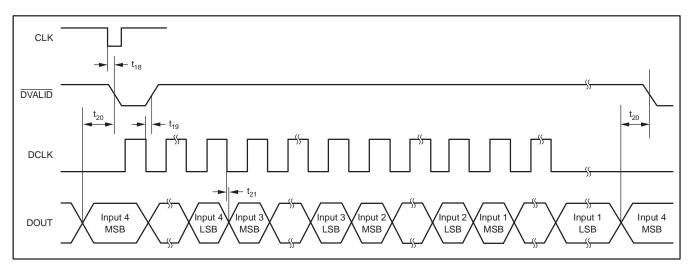
Figure 21. Digital Interface Timing Diagram for Data Retrieval From a Single DDC114
