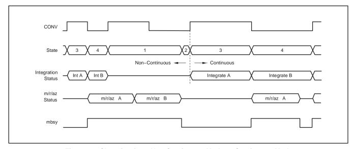
Figure 19. Changing from Non-Continuous Mode to Continuous Mode
