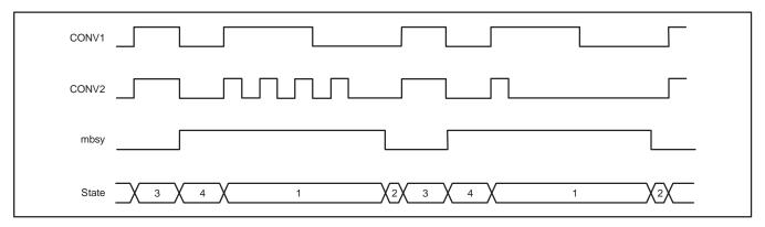
Figure 16. Equivalent CONV Signals in the Non-Continuous Mode
