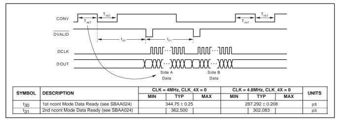
Figure 26. Readback in Non-Continuous Mode
