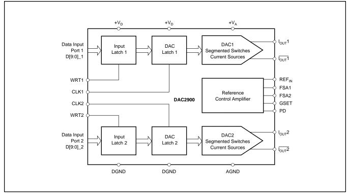
FIGURE 1. Block Diagram of the DAC2900.
