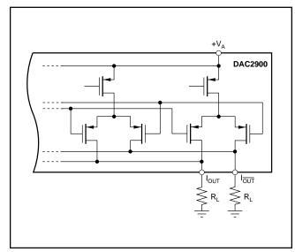
FIGURE 2. Equivalent Analog Output.
