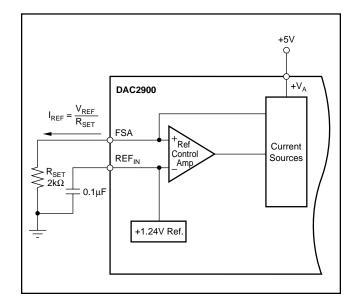
FIGURE 7. Internal Reference Configuration.
