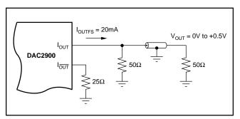
FIGURE 6. Driving a Doubly Terminated 50ý Cable Directly.
