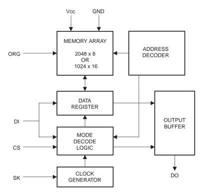
Note: 1. When the ORG pin is connected to Vcc, the x 16 organization is selected. When it is connected to ground, the x 8 organization is selected. If the ORG pin is left unconnected and the application does not load the input beyond the capability of the internal 1 Meg ohm pullup, then the x 16 organization is selected. This feature is not available on the 1.8V devices.
