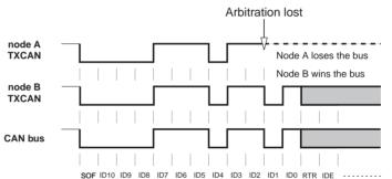
The CAN protocol handles bus accesses according to the concept called "Carrier Sense Multiple Access with Arbitration on Message Priority".
