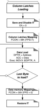
Note: The last page address used when loading the column latch is the one used to select the page programming address.
