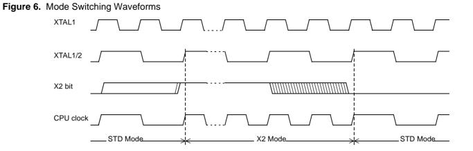
Note: In order to prevent any incorrect operation while operating in the X2 mode, users must be aware that all peripherals using the clock frequency as a time reference (UART, timers...) will have their time reference divided by two. For example a free running timer generating an interrupt every 20 ms will then generate an interrupt every 10 ms. A UART with a 4800 baud rate will have a 9600 baud rate.
