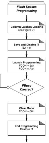
Figure 22. Flash and Extra Row Programming Procedure
