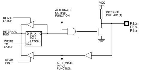
Note: The internal pull-up can be disabled on P1 when analog function is selected.
