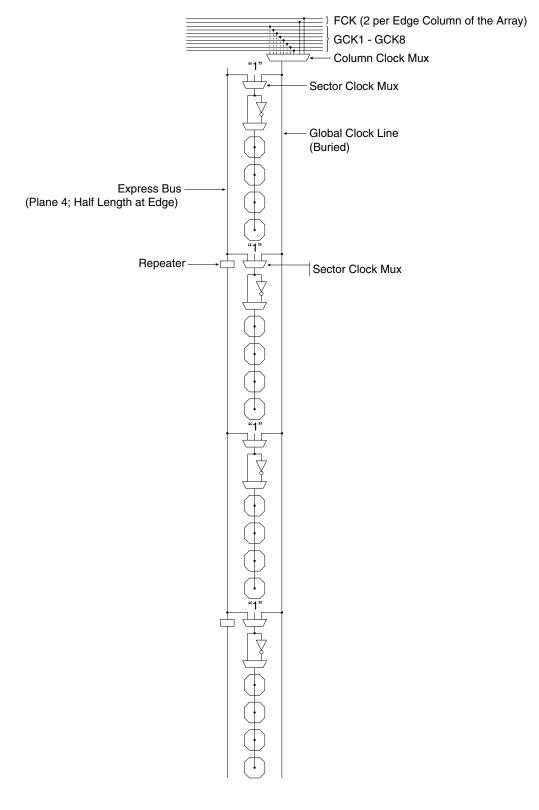
Figure 10. Clocking (for One Column of Cells)
