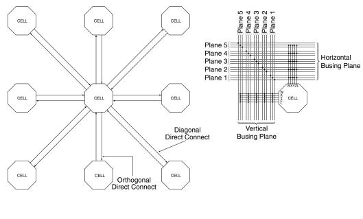
(a) Cell-to-cell Connections
