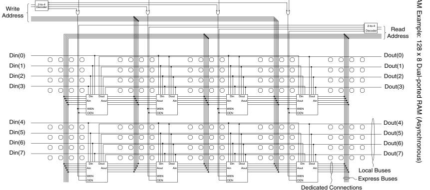
Figure 9. RAM Example: 128 x 8 Dual-ported RAM (Asynchronous)
