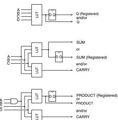
Synthesis Mode. This mode is particularly important for the use of VHDL/Verilog design. VHDL/Verilog Synthesis tools generally will produce as their output large amounts of random logic functions. Having a 4-input LUT structure gives efficient random logic optimization without the delays associated with larger LUT structures. The output of any cell may be registered, tri-stated and/or fed back into a core cell.
