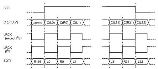
Figure 1. Audio routing mode timing (AKMODE=0)
