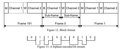
The sub-frame is defined in Figure 14 below. Bits 0-3 of the sub-frame represent a preamble for synchronization. There are three preambles. The block preamble, B, is contained in the first sub-frame of Frame 0. The channel 1 preamble, M, is contained in the first sub-frame of all other frames. The channel 2 preamble, W, is contained in all of the second sub-frames.
