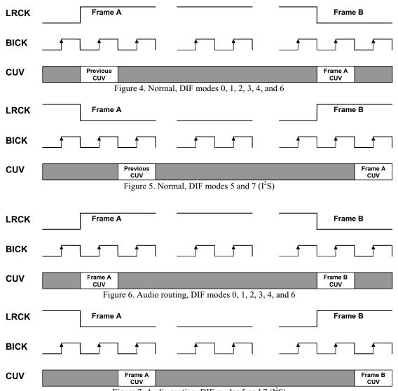
Figure 7. Audio routing, DIF modes 5 and 7 (I<sup>2</sup>S)
