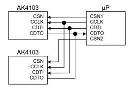
Figure 18. Typical connection with μP Note: External pull-up resistor should not be attached to CDTO pins since CDTO pin is internally connected to the pull-down resistor.
