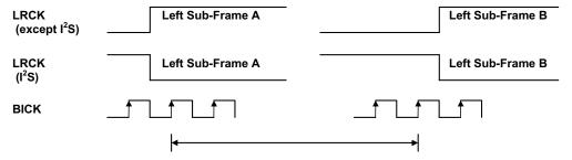
Figure 3. Block start timing in audio routing mode
