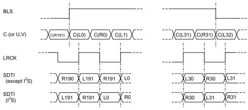
Figure 2. Audio routing mode timing (AKMODE=1)
