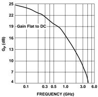
Figure 1. Power Gain vs. Frequency,  $I_d$  = 29 mA.
