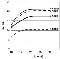
Figure 2. Power Gain vs. Current.
