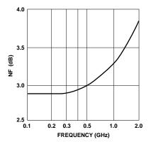
Figure 4. Noise Figure vs. Frequency,  $I_d$  = 29 mA.
