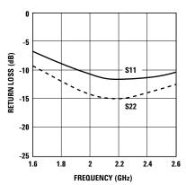
Figure 12. Input and Output return loss vs Frequency.
