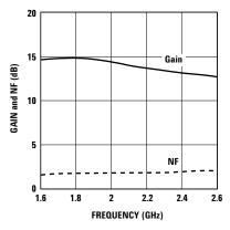
Figure 11. Gain and Noise Figure vs Frequency.
