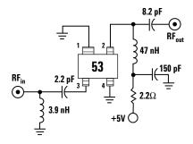
Figure 21. Schematic for 1900 MHz LNA design.
