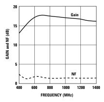
Figure 16. Gain and Noise Figure vs Frequency.
