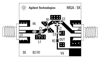
Figure 15. RF Layout for 1900 MHz HLA.
