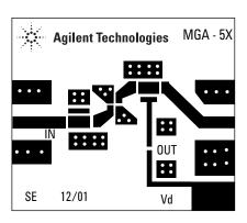
Figure 7. MGA-53453 PCB Layout.
