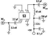
Figure 10. Schematic for a 1900 MHz stable circuit.
