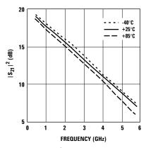
Figure 5.  $|S_{21}|^2$  vs. Frequency and Temperature.
