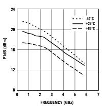
Figure 4. Output Power at 1dB Compression vs. Frequency and Temperature.
