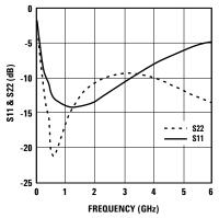
Figure 7. S11 and S22 (50 $\Omega$ ) vs. Frequency.
