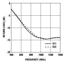
Figure 17. Input and Output return loss vs Frequency.
