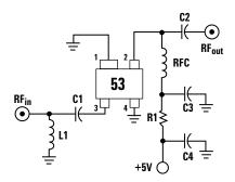
Figure 2. Schematic diagram with bias connections.
