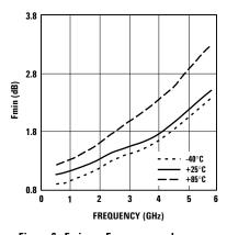
Figure 6. Fmin vs. Frequency and Temperature.
