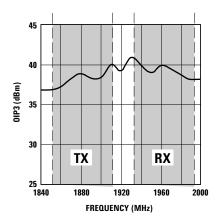
Figure 13. OIP3 vs. Frequency.
