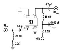
Figure 14. Schematic diagram for 900 MHz HLA.
