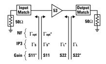
Figure 4. Definition of matching parameters.
