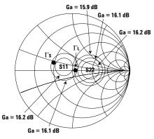
Figure 9. Input and output gain circles.
