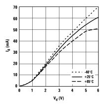
Figure 9. Current vs. Voltage and Temperature.
