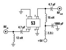
Figure 18. Schematic for 900 MHz LNA design.
