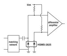
Figure 13. Differential Detector.
