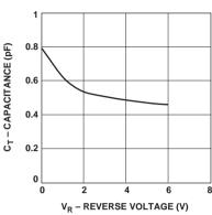
Figure 3. Total Capacitance vs. Reverse Voltage.
