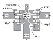
Figure 20. Layout of Suppressed Harmonic Detector.
