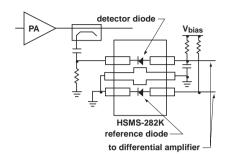
Figure 15. High Power Differential Detector.
