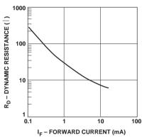
Figure 4. Dynamic Resistance vs. Forward Current.
