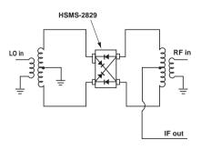
Figure 22. Planar Double Balanced Mixer.
