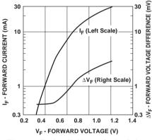
Figure 5. Typical  $V_{\rm f}$  Match, Series Pairs and Quads at Mixer Bias Levels.
