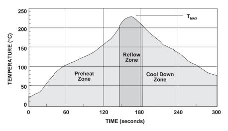
Figure 28. Surface Mount Assembly Profile.
