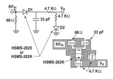
Figure 18. Temperature Compensated Detector.
