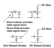
Figure 11. Single Diode Detectors.
