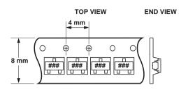
Note: "###" represents Package Marking Code. Package marking is right side up with carrier tape perforations at top. Conforms to Electronic Industries RS-481, "Taping of Surface Mounted Components for Automated Placement." Standard quantity is 3,000 devices per reel.
