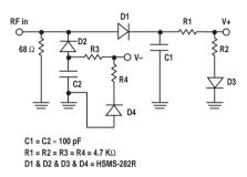
Figure 19. Schematic of Suppressed Harmonic Detector.
