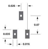
Figure 26. PCB Pad Layout, SOT-323 (dimensions in inches).
