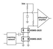
Figure 16. Voltage Doubler Differential Detector.
