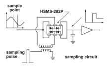
Figure 25. Sampling Circuit.
