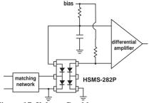
Figure 17. Voltage Doubler Differential Detector.
