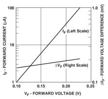
Figure 6. Typical  $V_{\rm f}$  Match, Series Pairs at Detector Bias Levels.
