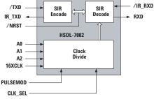
Figure 1. Block Diagram of HSDL-7002
