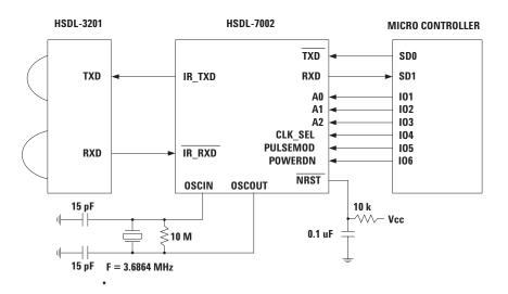
Note: POWERDN can be used as a basic chip select. The HSDL-7002 will not be able to receive or transmit data while POWERDN is asserted.
