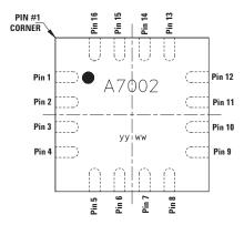
Figure 2. HSDL-7002 Pin Configuration
