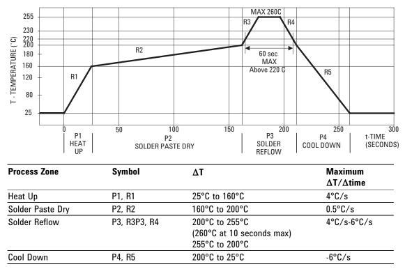
The reflow profile is a straight-line representation of a nominal temperature profile for a convective reflow solder process. The temperature profile is divided into four process zones, each with different DT/Dtime temperature change rates. The DT/Dtime rates are detailed in the above table. The temperatures are measured at the component to printed circuit board connections.
