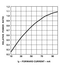
Figure 4. Normalized Transmitter Output Power vs. Forward Current.
