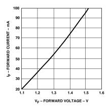
Figure 3. Typical Forward Voltage and Current Characteristics.
