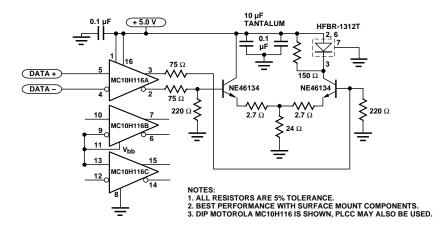
Figure 5. Recommended Transmitter Drive and Test Circuit.
