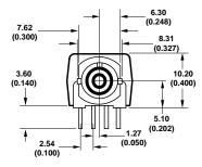
HFBR-2316T is pin compatible with HFBR-24X6 receivers and can be used to extend the distance of an existing application by substituting the HFBR-2316T for the HFBR-2416.
