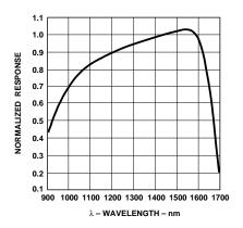
Figure 10. Normalized Receiver Spectral Response.
