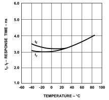
Figure 9. Typical Rise and Fall Times vs. Temperature.
