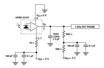
Figure 6. HFBR-2316T Receiver Test Circuit.
