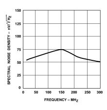
Figure 7. Typical Output Spectral Noise Density vs. Frequency.
