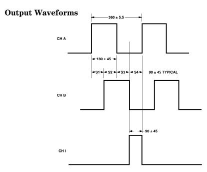
NOTE: ALL VALUES ARE IN ELECTRICAL DEGREES, WHERE  $360^\circ$  e = 1 CYCLE OF RESOLUTION. ERRORS ARE WORST CASE OVER ONE REVOLUTION. CH B LEADS CH A FOR COUNTERCLOCKWISE ROTATION. CH A LEADS CH B FOR CLOCKWISE ROTATION.
