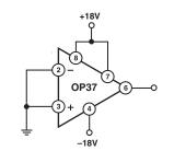
Figure 3. Burn-In Circuit
