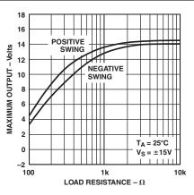
TPC 21. Maximum Output Voltage vs. Load Resistance
