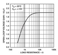
TPC 30. Open-Loop Voltage Gain vs. Load Resistance
