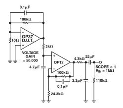
TPC 28. Noise Test Circuit (0.1 Hz to 10 Hz)
