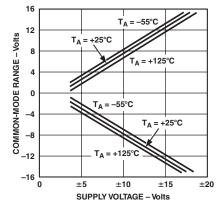
TPC 27. Common-Mode Input Range vs. Supply Voltage
