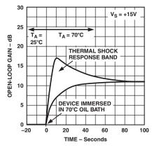
TPC 13. Offset Voltage Change Due to Thermal Shock
