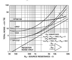
Figure 7. !0 Hz Noise vs. Source resistance (InIcludes Resistor Noise)
