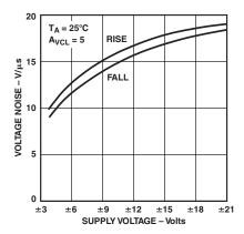
TPC 33. Slew Rate vs. Supply Voltage
