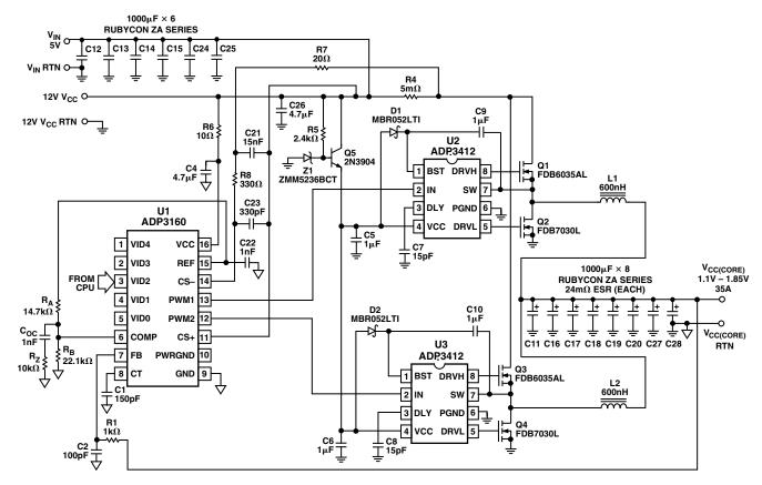
Figure 4. 35 A Athlon CPU Supply Circuit
