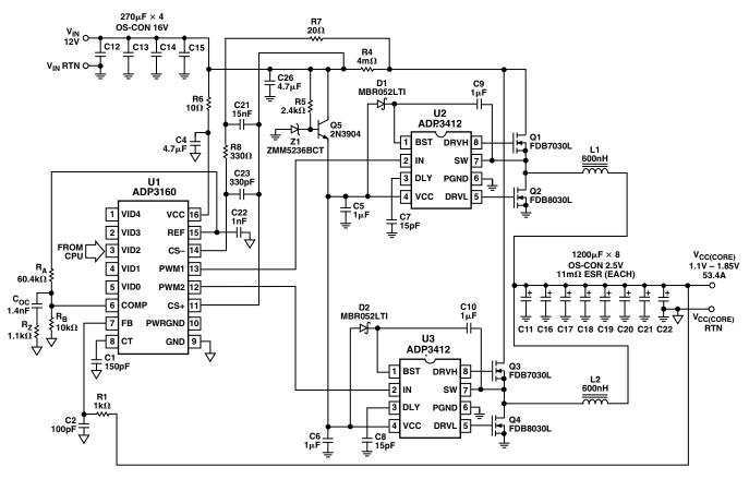
Figure 3. 53.4 A Intel CPU Supply Circuit
