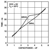
TPC 6. DRVH and DRVL Fall Times vs. Load Capacitance
