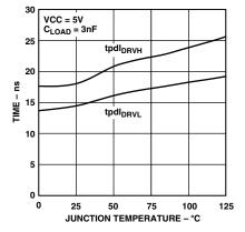
TPC 7. Propagation Delay vs. Temperature
