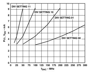
Figure 19. PLLVDD vs. f<sub>DAC</sub>
