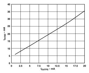
Figure 17. I<sub>AVDD</sub> vs. I<sub>OUTFS</sub>
