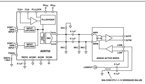
Figure 30. QAM Transmitter Architecture Using AD9755 and AD8343 Active Mixer
