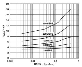
Figure 18. I<sub>DVDD</sub> vs. f<sub>OUT</sub>/f<sub>DAC</sub> Ratio
