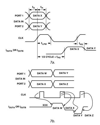
Figure 7. DAC Input Timing Requirements with PLL Active
