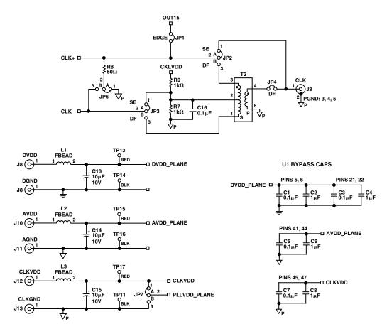
Figure 35. Evaluation Board Clock Circuitry
