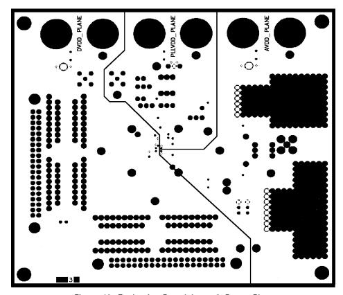
Figure 40. Evaluation Board, Layer 3, Power Plane
