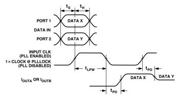
Figure 1. I/O Timing
