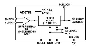
Figure 10. Clock Circuitry with PLL Disabled
