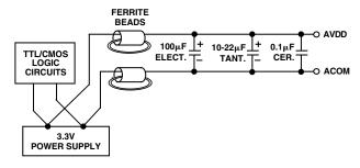
Figure 26. Differential LC Filter for a Single 3.3 V Application
