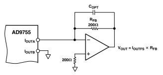
Figure 24. Unipolar Buffered Voltage Output
