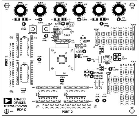
Figure 36. Evaluation Board, Assembly-Top
