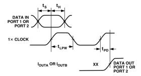
Figure 13. Timing Requirements, Noninterleaved Mode with PLL Disabled
