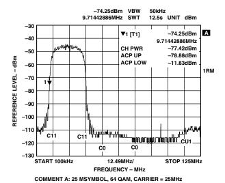
Figure 28. Reconstructed 64-QAM Signal at 25 MHz IF
