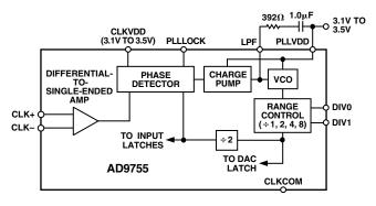
Figure 6. Clock Circuitry with PLL Active
