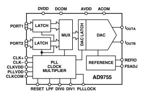
The DAC utilizes a segmented current source architecture combined with a proprietary switching technique to reduce glitch energy and to maximize dynamic accuracy. Differential current outputs support single-ended or differential applications. The differential outputs each provide a nominal full-scale current from 2 mA to 20 mA.
