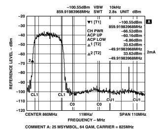
Figure 31. Signal of Figure 28 Mixed to Carrier Frequency of 800 MHz
