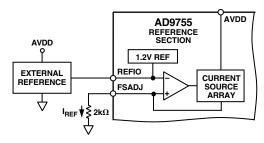
Figure 5. External Reference Configuration
