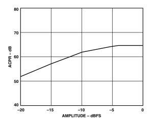
Figure 29. ACPR vs. Amplitude for QAM Carrier
