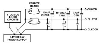
Figure 9. LC Network for Power Filtering
