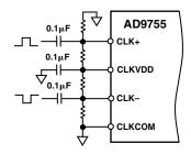
Figure 15b. Differential Clock Interface
