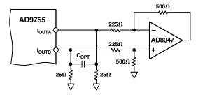
Figure 21. DC Differential Coupling Using an Op Amp
