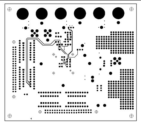
Figure 41. Evaluation Board, Bottom Layer
