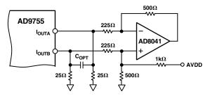
Figure 22. Single Supply DC Differential Coupled Circuit
