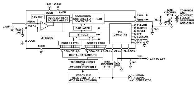
Figure 2. Basic AC Characterization Test Setup
