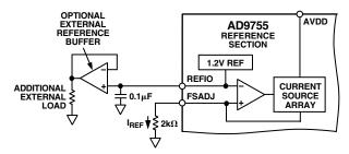
Figure 4. Internal Reference Configuration
