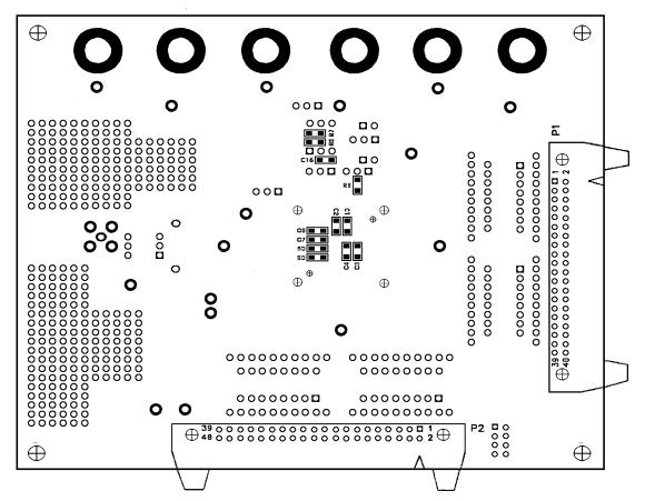
Figure 37. Evaluation Board, Assembly - Bottom
