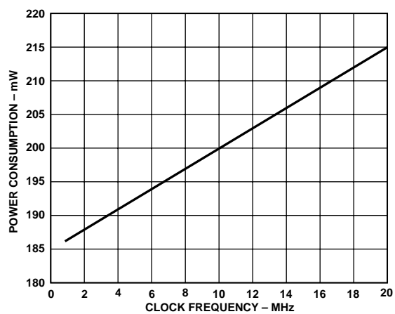
Figure 11. Power Consumption vs. Clock Frequency
